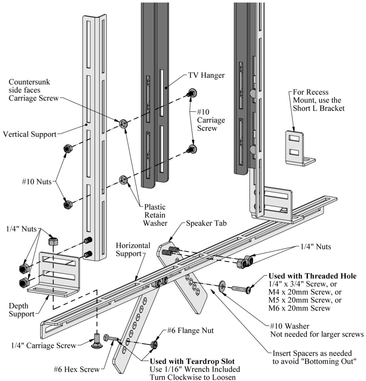
**Figure 1 Setup for a Speaker Below the TV**
